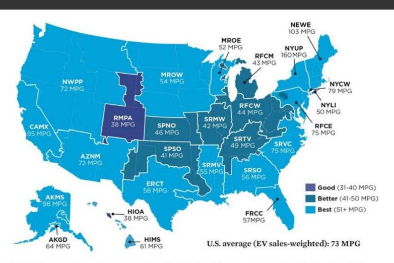
MPG, by region, needed for a gasoline vehicle to match an EV charged from the grid in 2014.
